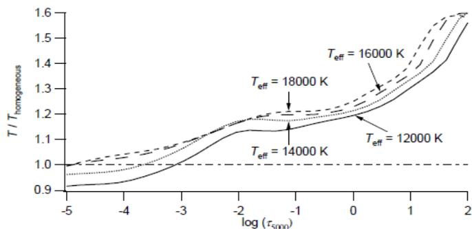
**Figure 1.** The ratio of the temperature as a function of optical depth in various models including stratification to that of a chemically homogeneous model with metallicity of -1.5 dex solar of the same effective temperature and surface gravity. The dotted-dashed line shows the position of a ratio of one.
