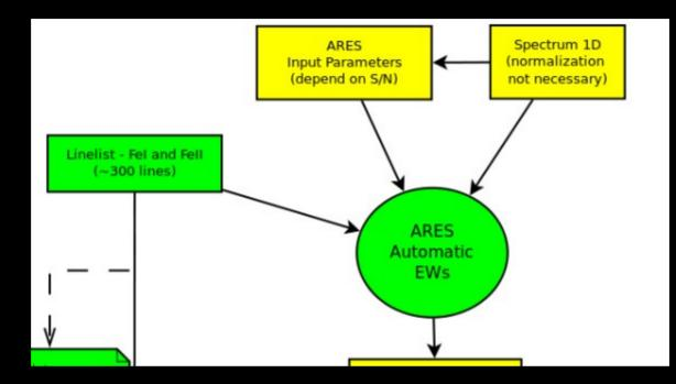
The first step is to determine the EWs for the iron lines.
